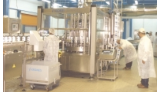
The application of sleeve labels to the plastic bottles is carried out on a Krones Sleeveomatic machine
