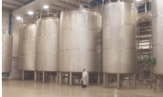
Located right beside the milk treatment department, the process milk tanks can hold up to 335,000 litres
